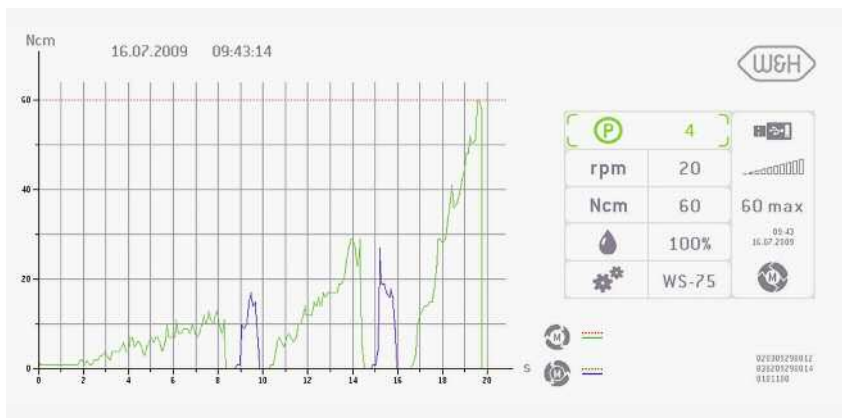
Recording of torque for a treatment step, including the parameters set
